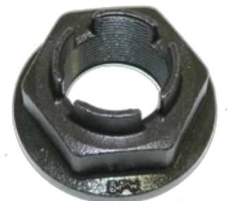
AXLE TYPE CB1505 PART # 02.5273.38.00 STUB AXLE SIZE M27 x 1.5 TORQUE 330Nm
