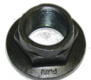
AXLE TYPE : CB854-CB1355 PART # 02.5273.36.00 STUB AXLE SIZE M24 x 1.5 TORQUE 280Nm
