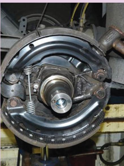
4. The new brake shoes are positioned and located with a soft hammer. Anchor retaining springs are re-fastened.
