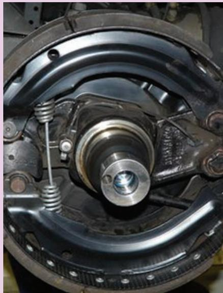
2. To dismantle, the brake shoes are simply levered off.
