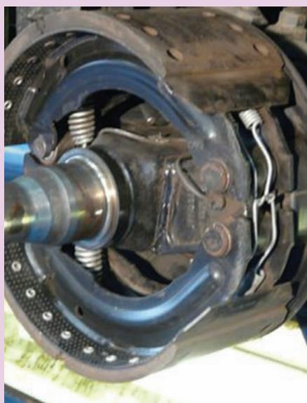
1. Anchor retaining springs in position
